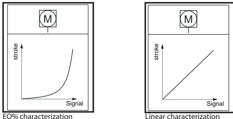
The actuator stroke can be selected via the Jumper and can be set to 2.5mm - 5.0mm or 5.5 mm
