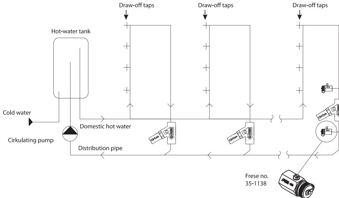
*It is recommendable to install pressure test points on both sides of the critical CirCon<sup>+</sup> valve in the installation for the verification of differential pressure.*
