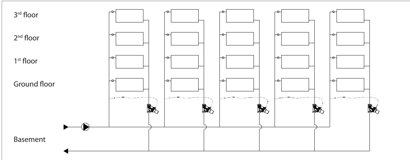
In this case the purpose of Frese PV Compact is to maintain pressure of approx. 12 kPa across the supply and the return line. Specifying the characteristics of the building, the calorific requirement was rated at 125 l/h per flat.
