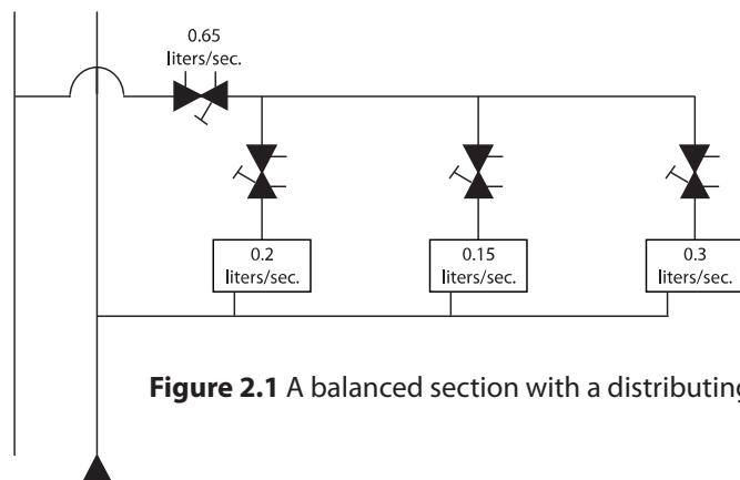
**Figure 2.1** A balanced section with a distributing line for three terminals.
