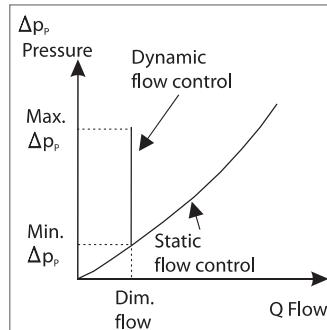
The differential pressure unit of the valve will work as soon as the differential pressure provided by the pump is sufficient. Consequently, the rated flow is maintained regardless of any pressure fluctuations in the system.
