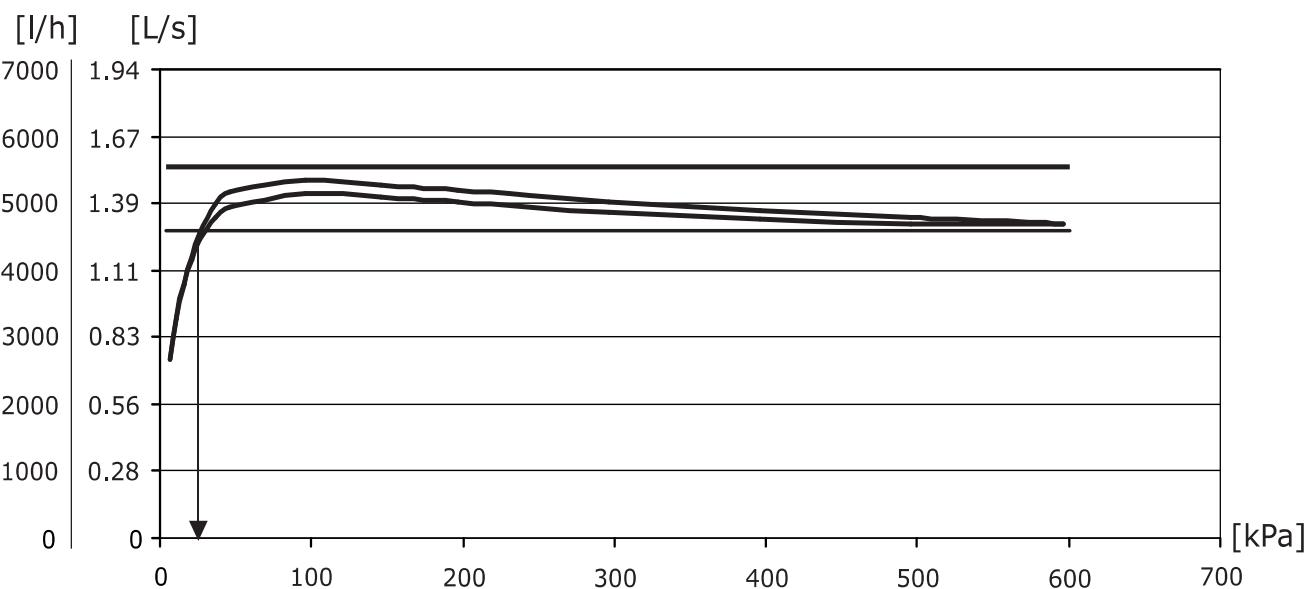
*Schematic view of the flow development for cartridge type 40, Frese no. 49-44176. Nominal flow 1.388 l/s / 4.816 l/h.
