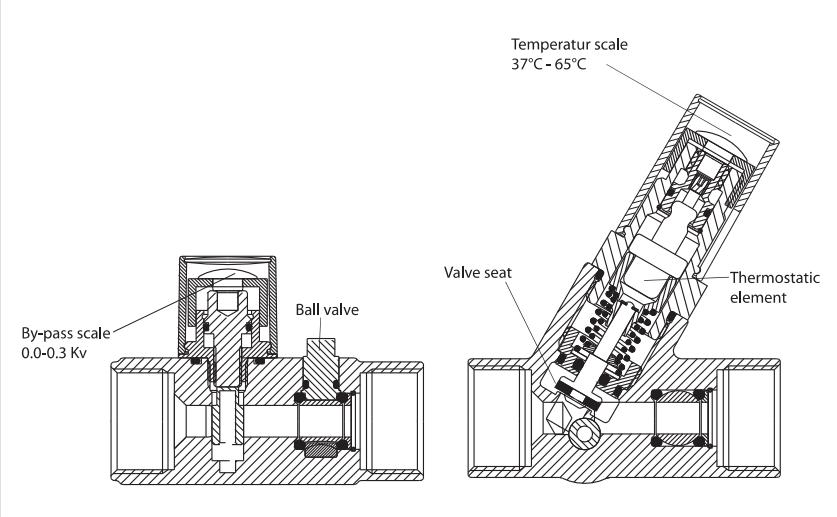
Section drawing of TemCon<sup>+</sup> DN20 fem./fem. with ball valve
