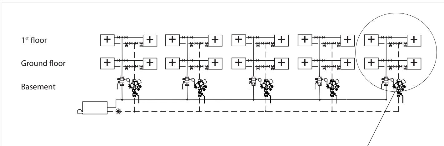
Evidently the pressure will be higher in the supply pipes near the pump than e.g. in the critical pipe.
